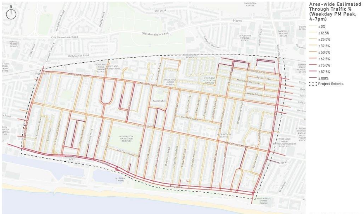
Figure 3-6: Flow Telematics Output showing Through-Traffic (%): 4-7pm
